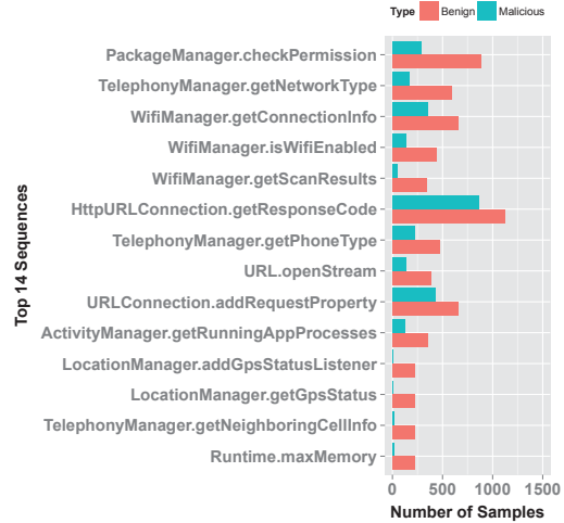
Figure 5: Top 14 differences of sensitive API calls between benign and malicious apps by 3,032 benign and malicious samples
