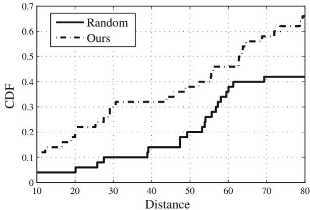
**Fig. 4** CDF of the distance between the actor and a sensor node detecting the event in a large-sized area
