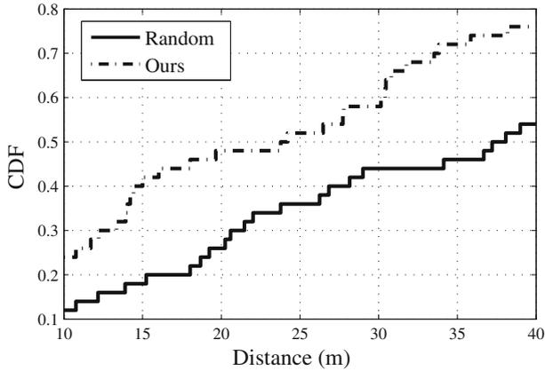
**Fig. 2** CDF of the distance between the actor and a sensor node detecting the event in a small-sized area
