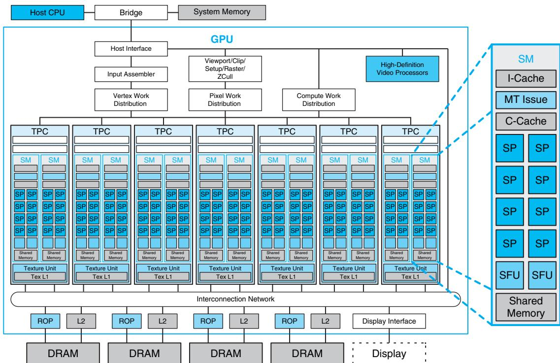
**FIGURE A.2.5 Basic unified GPU architecture.** Example GPU with 112 streaming processor (SP) cores organized in 14 streaming multiprocessors (SMs); the cores are highly multithreaded. It has the basic Tesla architecture of an NVIDIA GeForce 8800. The processors connect with four 64-bit-wide DRAM partitions via an interconnection network. Each SM has eight SP cores, two special function units (SFUs), instruction and constant caches, a multithreaded instruction unit, and a shared memory.
