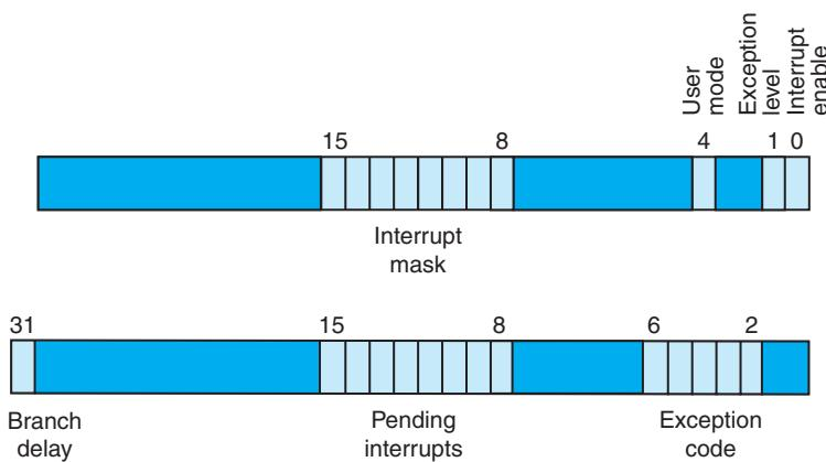
**FIGURE 6.11 The Cause and Status registers.** This version of the Cause register corresponds to the MIPS-32 architecture. The earlier MIPS I architecture had three nested sets of kernel/user and interrupt enable bits to support nested interrupts. [Section B.7 in Appendix B](#) has more details about these registers.
