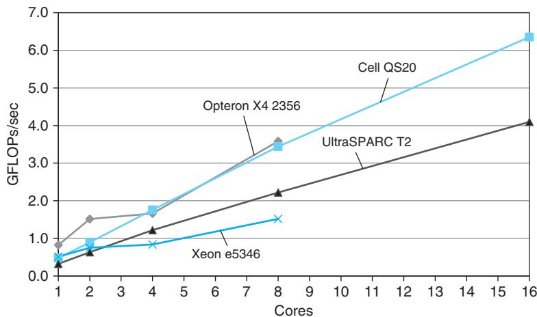
**FIGURE 7.20 Performance of SpMV on the four multicores.**
