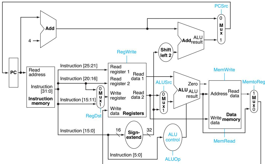
**FIGURE 4.15** The datapath of Figure 4.11 with all necessary multiplexors and all control lines identified. The control lines are shown in color. The ALU control block has also been added. The PC does not require a write control, since it is written once at the end of every clock cycle; the branch control logic determines whether it is written with the incremented PC or the branch target address.
