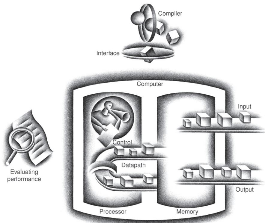
**FIGURE 1.4 The organization of a computer, showing the five classic components.** The processor gets instructions and data from memory. Input writes data to memory, and output reads data from memory. Control sends the signals that determine the operations of the datapath, memory, input, and output.
