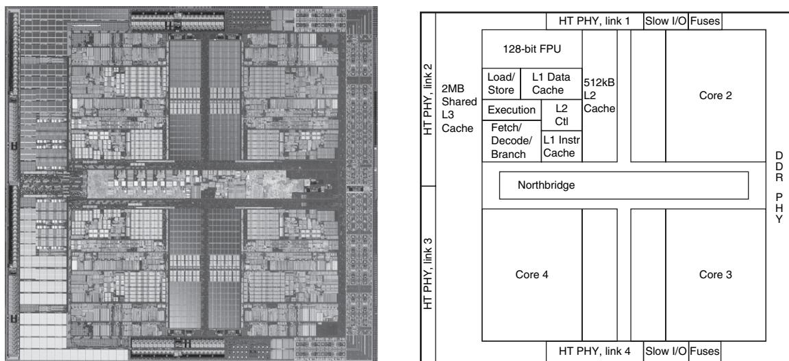
**FIGURE 1.9 Inside the AMD Barcelona microprocessor.** The left-hand side is a microphotograph of the AMD Barcelona processor chip, and the right-hand side shows the major blocks in the processor. This chip has four processors or “cores”. The microprocessor in the laptop in Figure 1.7 has two cores per chip, called an Intel Core 2 Duo.
