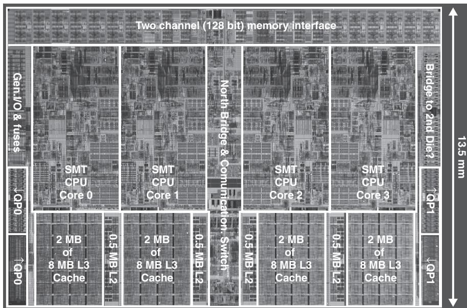
**FIGURE 5.37 An Intel Nehalem die processor photo with the components labeled.** This 13.5 by 19.6 mm die has 731 million transistors. It contains four processors that each have private 32-KB instruction and 32-LKB instruction caches and a 512-KB L2 cache. The four cores share an 8-MB L3 cache. The two 128-bit memory channels are to DDR3 DRAM. Each core also has a two-level TLB. The memory controller is now on the die, so there is no separate north bridge chip as in Intel Clovertown.
