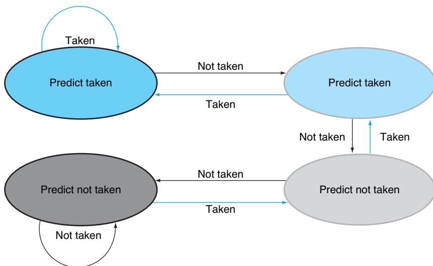
**FIGURE 4.63 The states in a 2-bit prediction scheme.** By using 2 bits rather than 1, a branch that strongly favors taken or not taken—as many branches do—will be mispredicted only once. The 2 bits are used to encode the four states in the system. The 2-bit scheme is a general instance of a counter-based predictor, which is incremented when the prediction is accurate and decremented otherwise, and uses the midpoint of its range as the division between taken and not taken.
