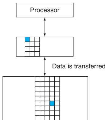
**FIGURE 5.2 Every pair of levels in the memory hierarchy can be thought of as having an upper and lower level.** Within each level, the unit of information that is present or not is called a *block* or a *line*. Usually we transfer an entire block when we copy something between levels.
