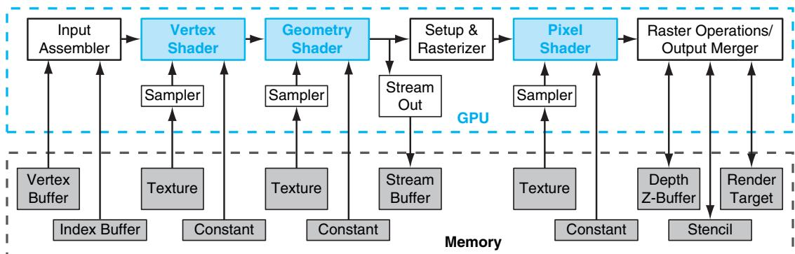
**FIGURE A.3.1 Direct3D 10 graphics pipeline.** Each logical pipeline stage maps to GPU hardware or to a GPU processor. Programmable shader stages are blue, fixed-function blocks are white, and memory objects are grey. Each stage processes a vertex, geometric primitive, or pixel in a streaming dataflow fashion.
