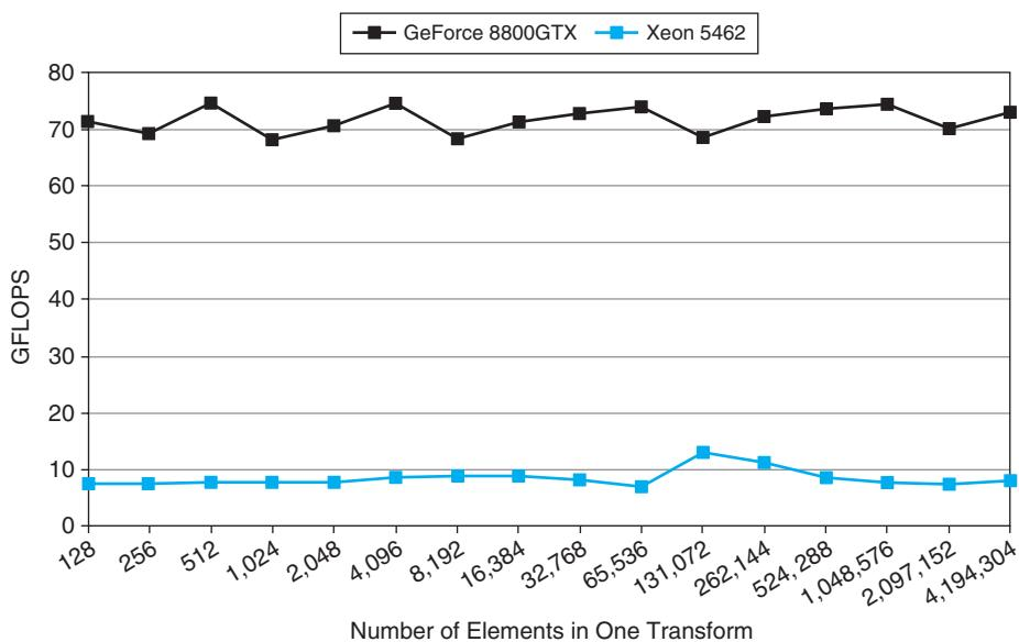
**FIGURE A.7.5 Fast Fourier Transform throughput performance.** The graph compares the performance of batched one-dimensional in-place complex FFTs on a 1.35 GHz GeForce 8800 GTX with a quad-core 2.8 GHz Intel Xeon E5462 series (code named “Harpertown”), 6MB L2 Cache, 4GB Memory, 1600 FSB, Red Hat Linux, Intel MKL 10.0.
