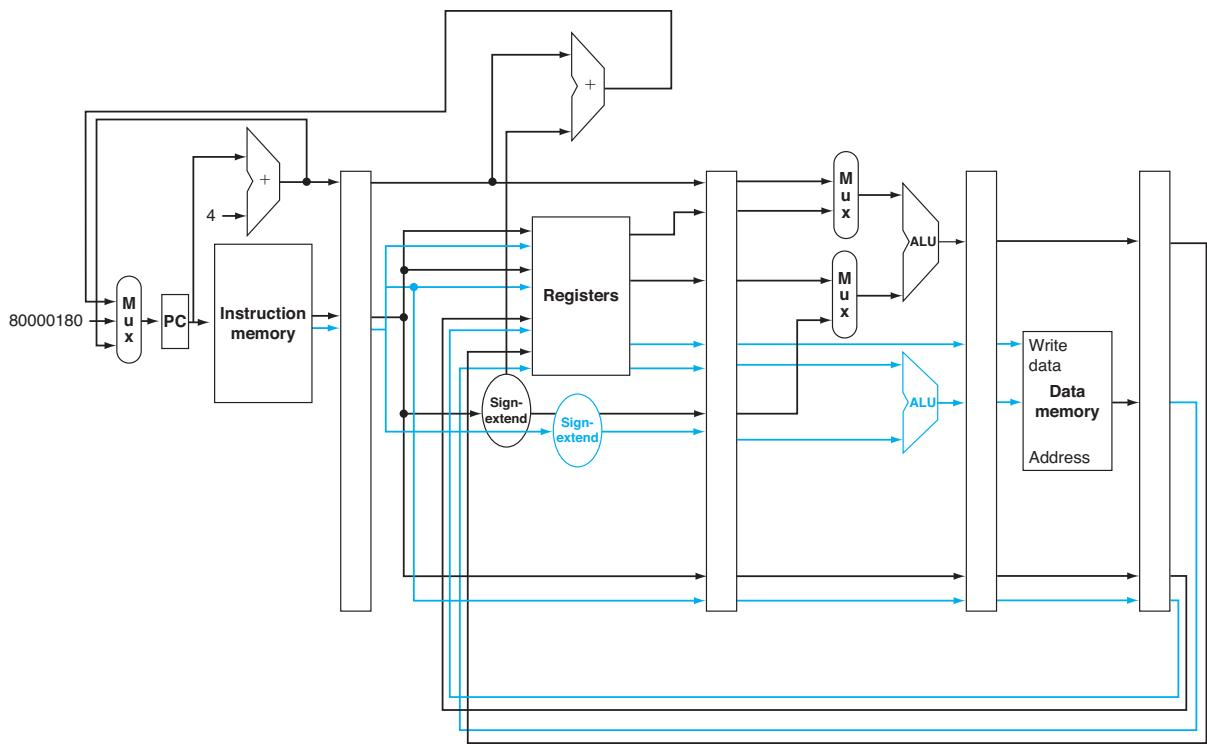
**FIGURE 4.69 A static two-issue datapath.** The additions needed for double issue are highlighted: another 32 bits from instruction memory, two more read ports and one more write port on the register file, and another ALU. Assume the bottom ALU handles address calculations for data transfers and the top ALU handles everything else.
