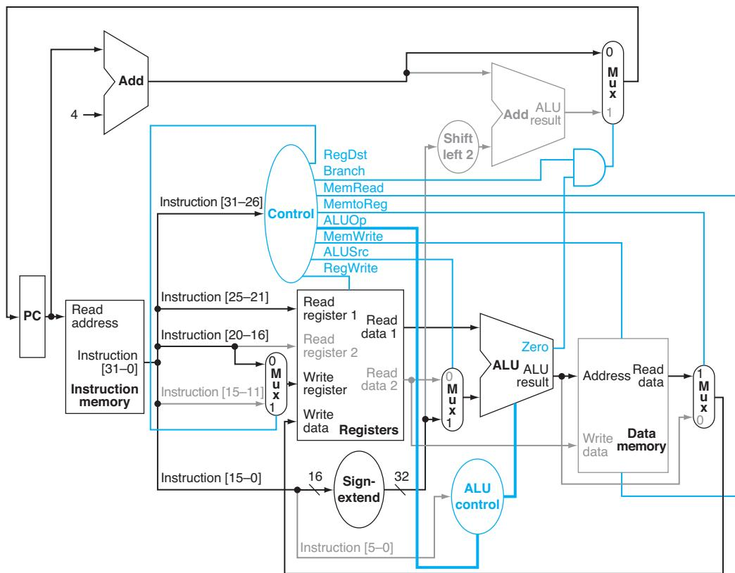
**FIGURE 4.20 The datapath in operation for a load instruction.** The control lines, datapath units, and connections that are active are highlighted. A store instruction would operate very similarly. The main difference would be that the memory control would indicate a write rather than a read, the second register value read would be used for the data to store, and the operation of writing the data memory value to the register file would not occur.
