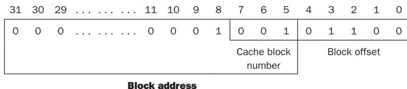
Byte address 300 is block address
