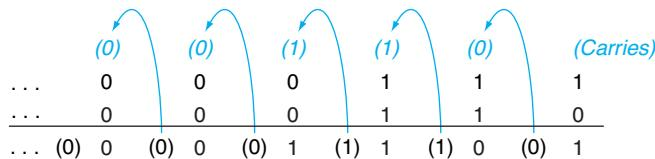
**FIGURE 3.1 Binary addition, showing carries from right to left.** The rightmost bit adds 1 to 0, resulting in the sum of this bit being 1 and the carry out from this bit being 0. Hence, the operation for the second digit to the right is  $0 + 1 + 1$ . This generates a 0 for this sum bit and a carry out of 1. The third digit is the sum of  $1 + 1 + 1$ , resulting in a carry out of 1 and a sum bit of 1. The fourth bit is  $1 + 0 + 0$ , yielding a 1 sum and no carry.
