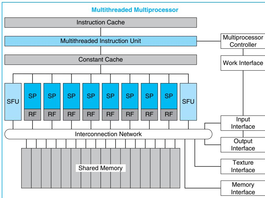
**FIGURE A.4.1 Multithreaded multiprocessor with eight scalar processor (SP) cores.** The eight SP cores each have a large multithreaded register file (RF) and share an instruction cache, multithreaded instruction issue unit, constant cache, two special function units (SFUs), interconnection network, and a multibank shared memory.
