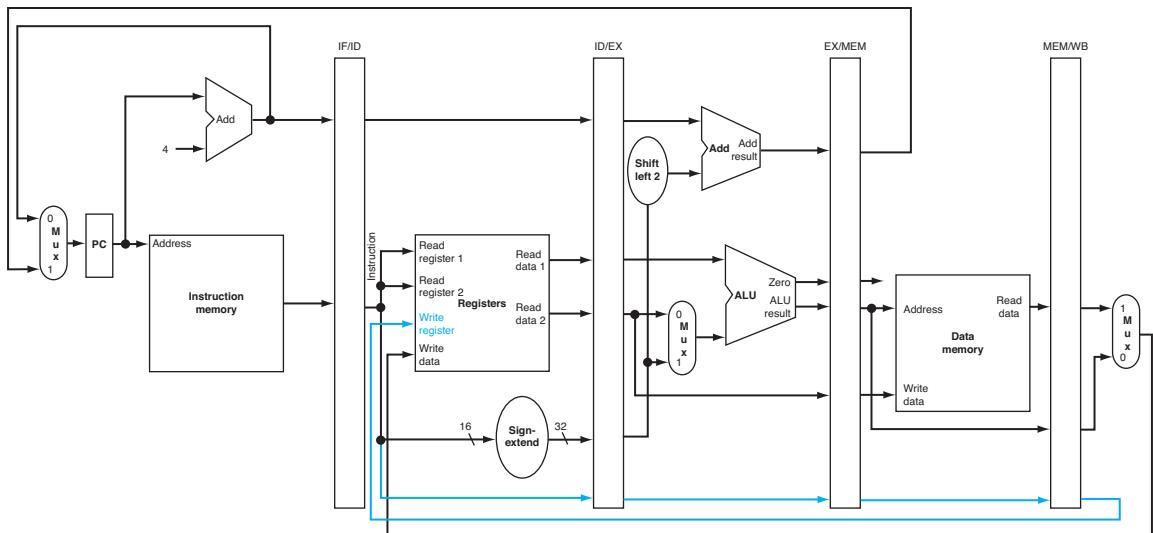
**FIGURE 4.41** The corrected pipelined datapath to handle the load instruction properly. The write register number now comes from the MEM/WB pipeline register along with the data. The register number is passed from the ID pipe stage until it reaches the MEM/WB pipeline register, adding five more bits to the last three pipeline registers. This new path is shown in color.
