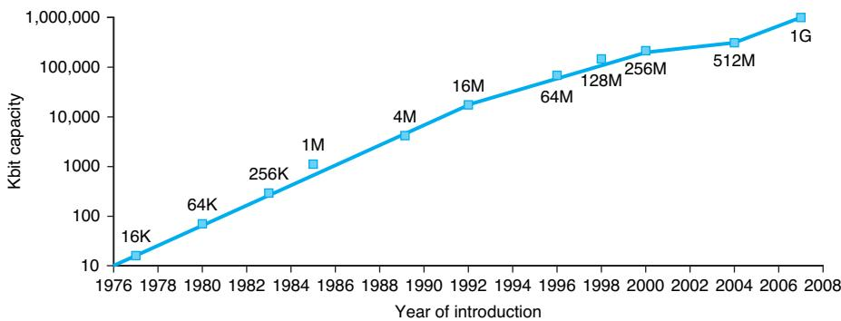
**FIGURE 1.12 Growth of capacity per DRAM chip over time.** The  $y$ -axis is measured in Kilobits, where  $K = 1024 (2^{10})$ . The DRAM industry quadrupled capacity almost every three years, a 60% increase per year, for 20 years. In recent years, the rate has slowed down and is somewhat closer to doubling every two years to three years.
