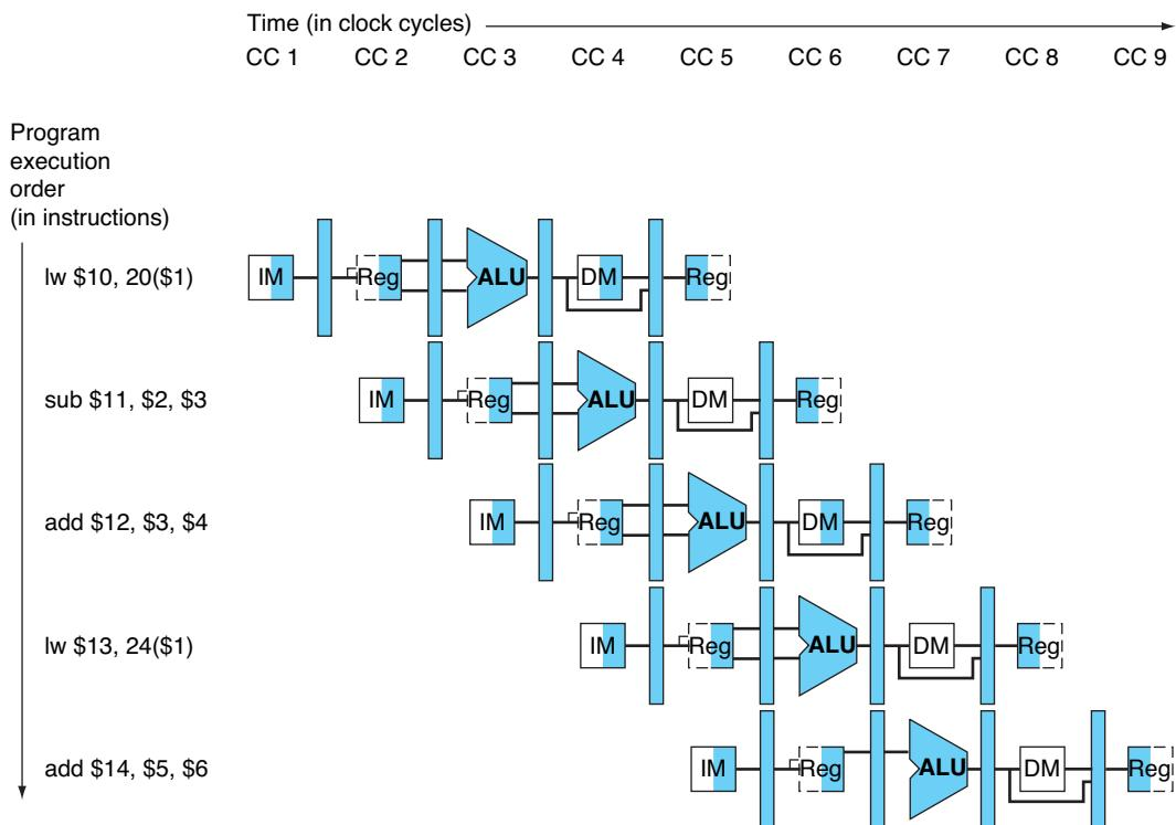
**FIGURE 4.43** **Multiple-clock-cycle pipeline diagram of five instructions.** This style of pipeline representation shows the complete execution of instructions in a single figure. Instructions are listed in instruction execution order from top to bottom, and clock cycles move from left to right. Unlike Figure 4.28, here we show the pipeline registers between each stage. Figure 4.44 shows the traditional way to draw this diagram.
