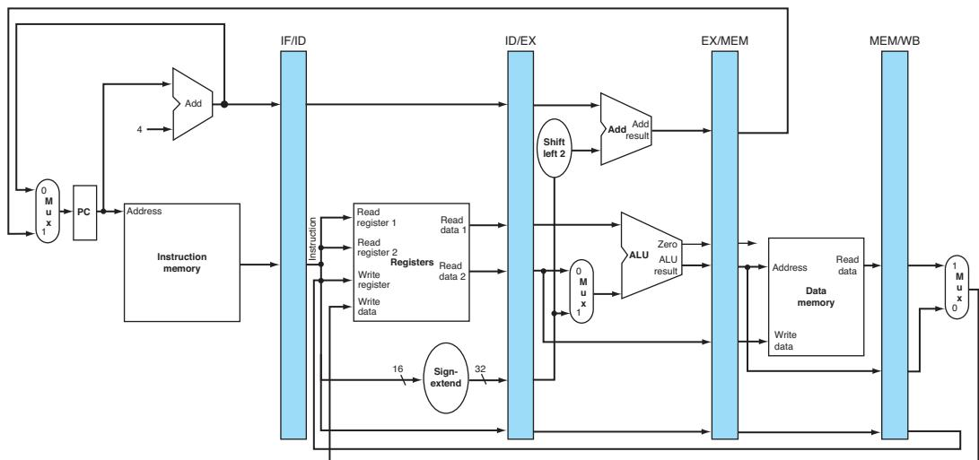
**FIGURE 4.45** The single-clock-cycle diagram corresponding to clock cycle 5 of the pipeline in Figures 4.43 and 4.44. As you can see, a single-clock-cycle figure is a vertical slice through a multiple-clock-cycle diagram.
