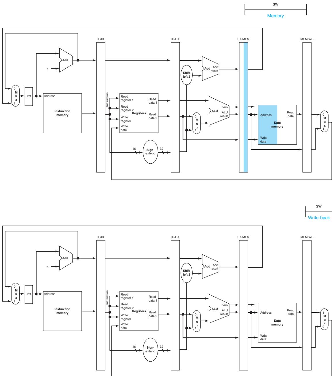
**FIGURE 4.40 MEM and WB: The fourth and fifth pipe stages of a store instruction.** In the fourth stage, the data is written into data memory for the store. Note that the data comes from the EX/MEM pipeline register and that nothing is changed in the MEM/WB pipeline register. Once the data is written in memory, there is nothing left for the store instruction to do, so nothing happens in stage 5.
