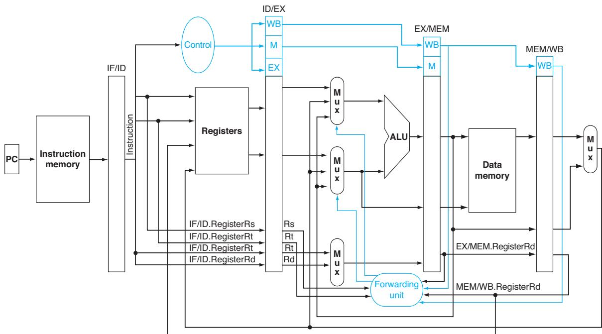
**FIGURE 4.56 The datapath modified to resolve hazards via forwarding.** Compared with the datapath in Figure 4.51, the additions are the multiplexors to the inputs to the ALU. This figure is a more stylized drawing, however, leaving out details from the full datapath, such as the branch hardware and the sign extension hardware.
