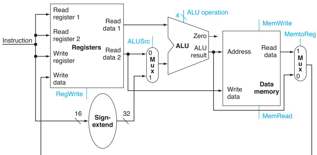
**FIGURE 4.10 The datapath for the memory instructions and the R-type instructions.** This example shows how a single datapath can be assembled from the pieces in [Figures 4.7](#) and [4.8](#) by adding multiplexors. Two multiplexors are needed, as described in the example.
