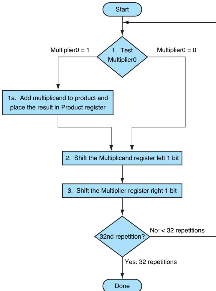
**FIGURE 3.5 The first multiplication algorithm, using the hardware shown in Figure 3.4.** If the least significant bit of the multiplier is 1, add the multiplicand to the product. If not, go to the next step. Shift the multiplicand left and the multiplier right in the next two steps. These three steps are repeated 32 times.
