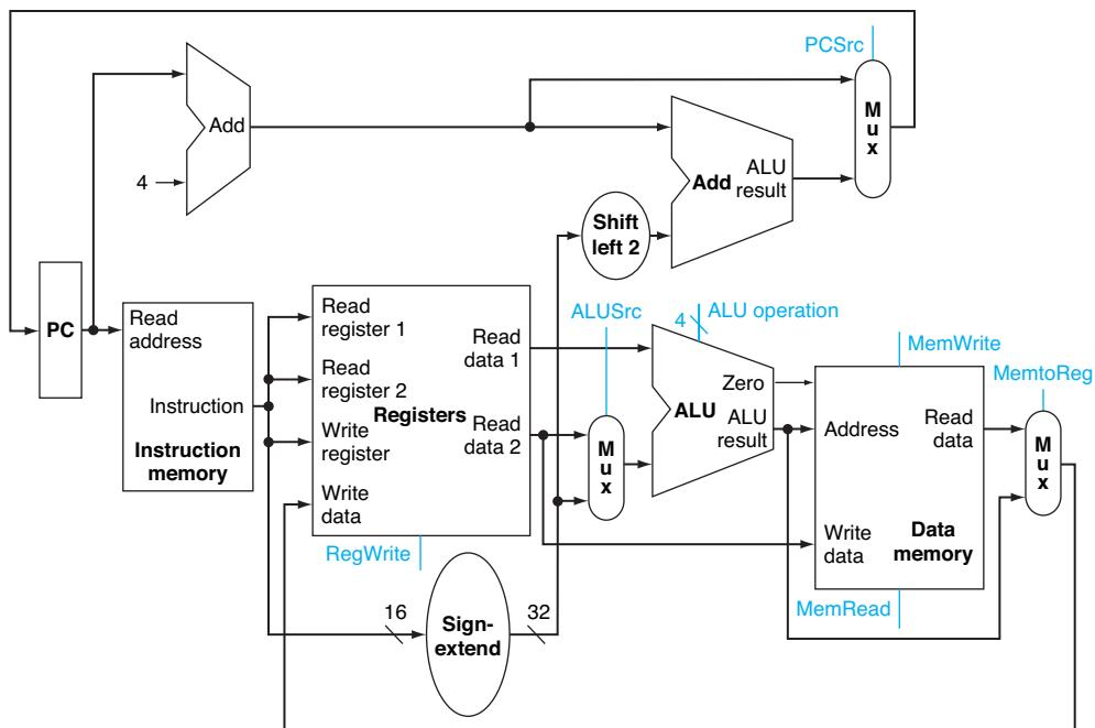
**FIGURE 4.11 The simple datapath for the MIPS architecture combines the elements required by different instruction classes.** The components come from Figures 4.6, 4.9, and 4.10. This datapath can execute the basic instructions (load-store word, ALU operations, and branches) in a single clock cycle. An additional multiplexor is needed to integrate branches. The support for jumps will be added later.
