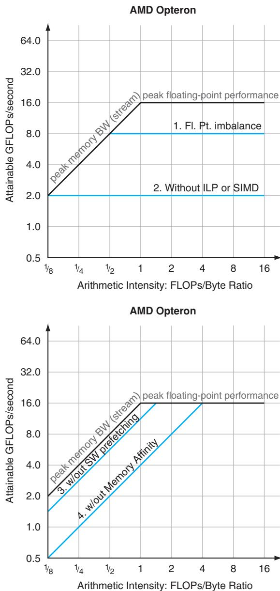
**FIGURE 7.15 Roofline model with ceilings.** The top graph shows the computational “ceilings” of 8 GFLOPs/sec if the floating-point operation mix is imbalanced and 2 GFLOPs/sec if the optimizations to increase ILP and SIMD are also missing. The bottom graph shows the memory bandwidth ceilings of 11 GB/sec without software prefetching and 4.8 GB/sec if memory affinity optimizations are also missing.
