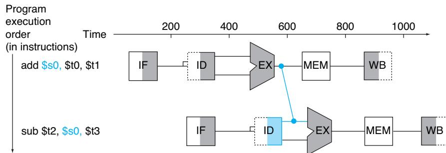
**FIGURE 4.29 Graphical representation of forwarding.** The connection shows the forwarding path from the output of the *EX* stage of *add* to the input of the *EX* stage for *sub*, replacing the value from register  $\$s0$  read in the second stage of *sub*.
