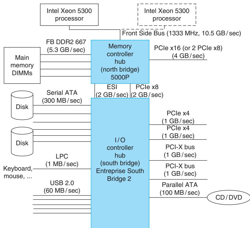
**FIGURE 6.9 Organization of the I/O system on an Intel server using the Intel 5000P chip set.** If you assume reads and writes are each half the traffic, you can double the bandwidth per link for PCIe.
