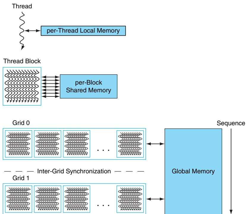
**FIGURE A.3.5 Nested granularity levels—thread, thread block, and grid—have corresponding memory sharing levels—local, shared, and global.** Per-thread local memory is private to the thread. Per-block shared memory is shared by all threads of the block. Per-application global memory is shared by all threads.
