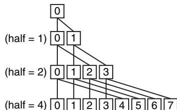
**FIGURE 7.3 The last four levels of a reduction that sums results from each processor, from bottom to top.** For all processors whose number *i* is less than half, add the sum produced by processor number (*i* + half) to its sum.
