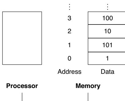
**FIGURE 2.2 Memory addresses and contents of memory at those locations.** If these elements were words, these addresses would be incorrect, since MIPS actually uses byte addressing, with each word representing four bytes. [Figure 2.3](#) shows the memory addressing for sequential word addresses.
