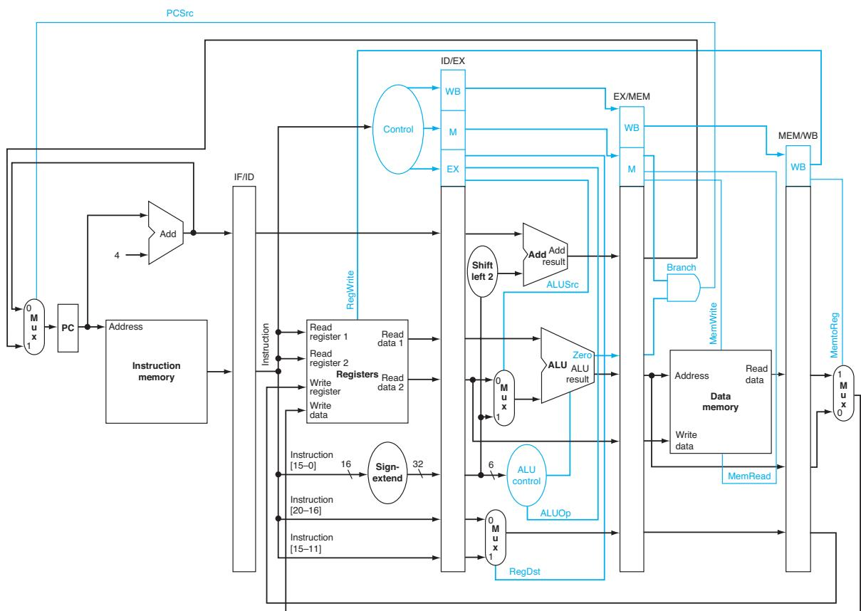
**FIGURE 4.51** The pipelined datapath of Figure 4.46, with the control signals connected to the control portions of the pipeline registers. The control values for the last three stages are created during the instruction decode stage and then placed in the ID/EX pipeline register. The control lines for each pipe stage are used, and remaining control lines are then passed to the next pipeline stage.
