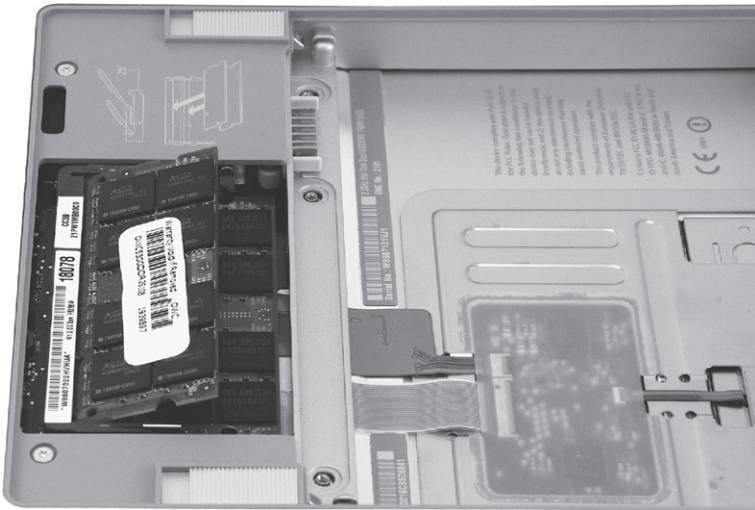
**FIGURE 1.8 Close-up of the bottom of the laptop reveals the memory.** The main memory is contained on one or more small boards shown on the left. The hole for the battery is to the right. The DRAM chips are mounted on these boards (called **DIMMs**, for dual inline memory modules) and then plugged into the connectors. Photo courtesy of OtherWorldComputing.com.
