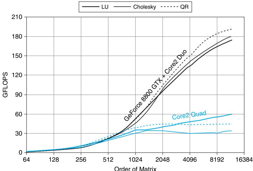
**FIGURE A.7.4 Dense matrix factorization performance rates.** The graph shows GFLOPS rates achieved in matrix factorizations using the GPU and using the CPU alone. Adapted from Figure 7 of Volkov and Demmel [2008]. The black lines are a 1.35 GHz NVIDIA GeForce 8800 GTX, CUDA 1.1, Windows XP attached to a 2.67 GHz Intel Core2 Duo E6700 Windows XP, including all CPU-GPU data transfer times. The blue lines are a quad-core 2.4 GHz Intel Core2 Quad Q6600, 64-bit Linux, Intel MKL 10.0.
