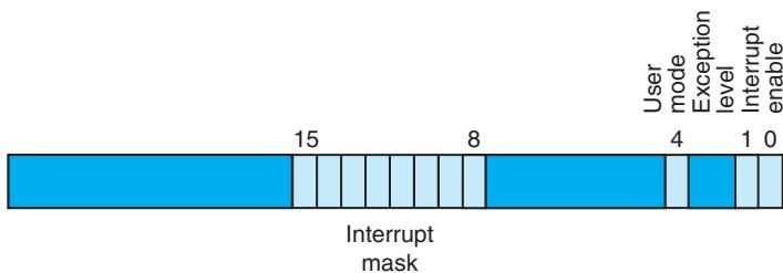
**FIGURE B.7.1** The Status register.
