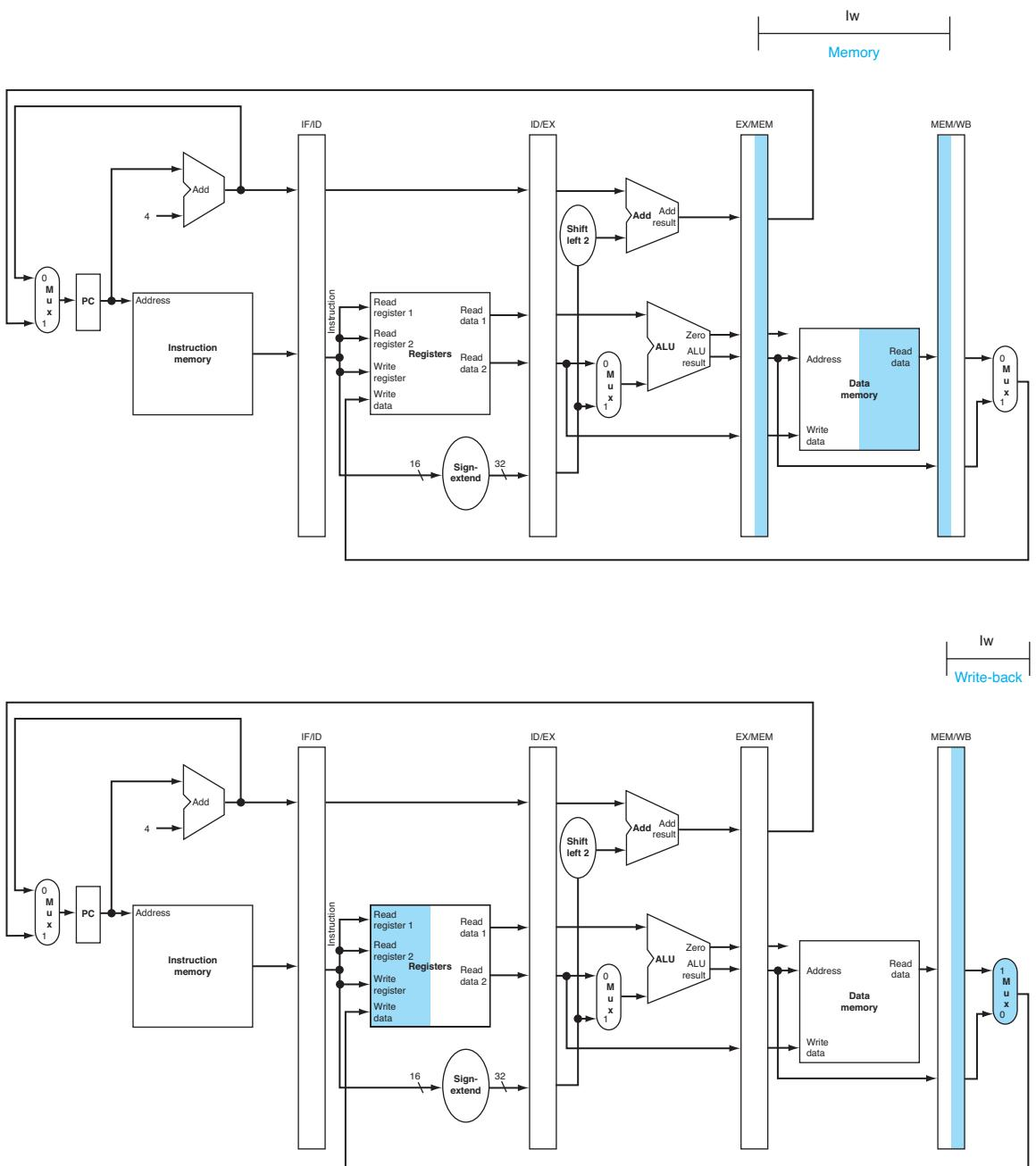
**FIGURE 4.38 MEM and WB: The fourth and fifth pipe stages of a load instruction, highlighting the portions of the datapath in Figure 4.35 used in this pipe stage.** Data memory is read using the address in the EX/MEM pipeline registers, and the data is placed in the MEM/WB pipeline register. Next, data is read from the MEM/WB pipeline register and written into the register file in the middle of the datapath. Note: there is a bug in this design that is repaired in Figure 4.41.
