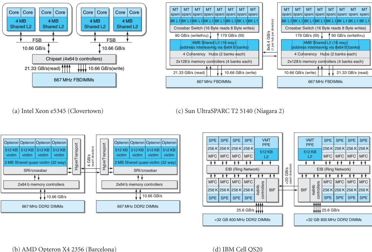
**FIGURE 7.17 Four recent multiprocessors, each using two sockets for the processors.** Starting from the upper left hand corner, the computers are: (a) Intel Xeon e5345 (Clovertown), (b) AMD Opteron X4 2356 (Barcelona), (c) Sun UltraSPARC T2 5140 (Niagara 2), and (d) IBM Cell QS20. Note that the Intel Xeon e5345 (Clovertown) has a separate north bridge chip not found in the other microprocessors.
