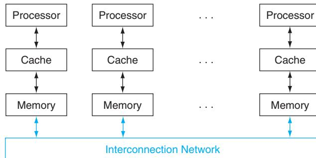
**FIGURE 7.4 Classic organization of a multiprocessor with multiple private address spaces, traditionally called a message-passing multiprocessor.** Note that unlike the SMP in Figure 7.2, the interconnection network is not between the caches and memory but is instead between processor-memory nodes.
