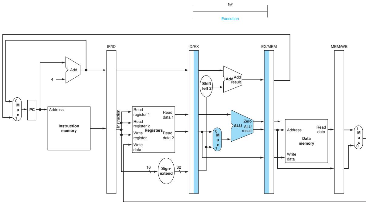
**FIGURE 4.39 EX: The third pipe stage of a store instruction.** Unlike the third stage of the load instruction in Figure 4.37, the second register value is loaded into the EX/MEM pipeline register to be used in the next stage. Although it wouldn't hurt to always write this second register into the EX/MEM pipeline register, we write the second register only on a store instruction to make the pipeline easier to understand.
