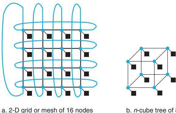
**FIGURE 7.9 Network topologies that have appeared in commercial parallel processors.**
