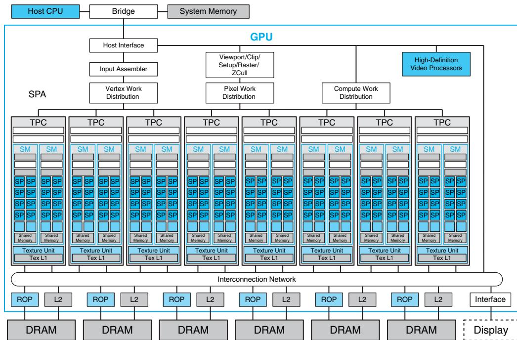
**FIGURE A.7.1 NVIDIA Tesla unified graphics and computing GPU architecture.** This GeForce 8800 has 128 streaming processor (SP) cores in 16 streaming multiprocessors (SMs), arranged in eight texture/processor clusters (TPC). The processors connect with six 64-bit-wide DRAM partitions via an interconnection network. Other GPUs implementing the Tesla architecture vary in the number of SP cores, SMs, DRAM partitions, and other units.
