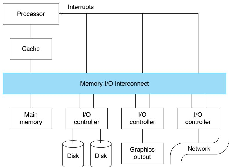
**FIGURE 6.1 A typical collection of I/O devices.** The connections between the I/O devices, processor, and memory are historically called *buses*, although the term means shared parallel wires and most I/O connections today are closer to dedicated serial lines. Communication among the devices and the processor uses both interrupts and protocols on the interconnect, as we will see in this chapter. Figure 6.9 shows the organization for a desktop PC.
