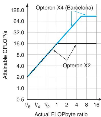
**FIGURE 7.14** **Rooftop models of two generations of Opterons.** The Opteron X2 rooftop, which is the same as Figure 7.11, is in black, and the Opteron X4 rooftop is in color. The larger rooftop point of Opteron X4 means that kernels that were computationally bound on the Opteron X2 could be memory-performance bound on the Opteron X4.
