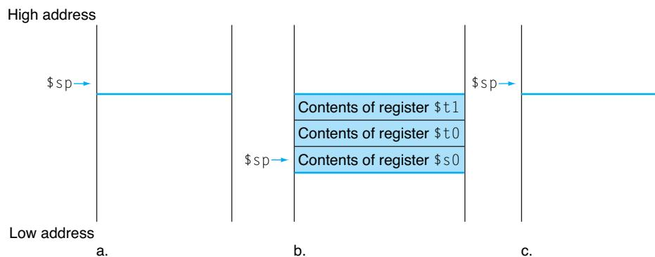
**FIGURE 2.10 The values of the stack pointer and the stack (a) before, (b) during, and (c) after the procedure call.** The stack pointer always points to the “top” of the stack, or the last word in the stack in this drawing.
