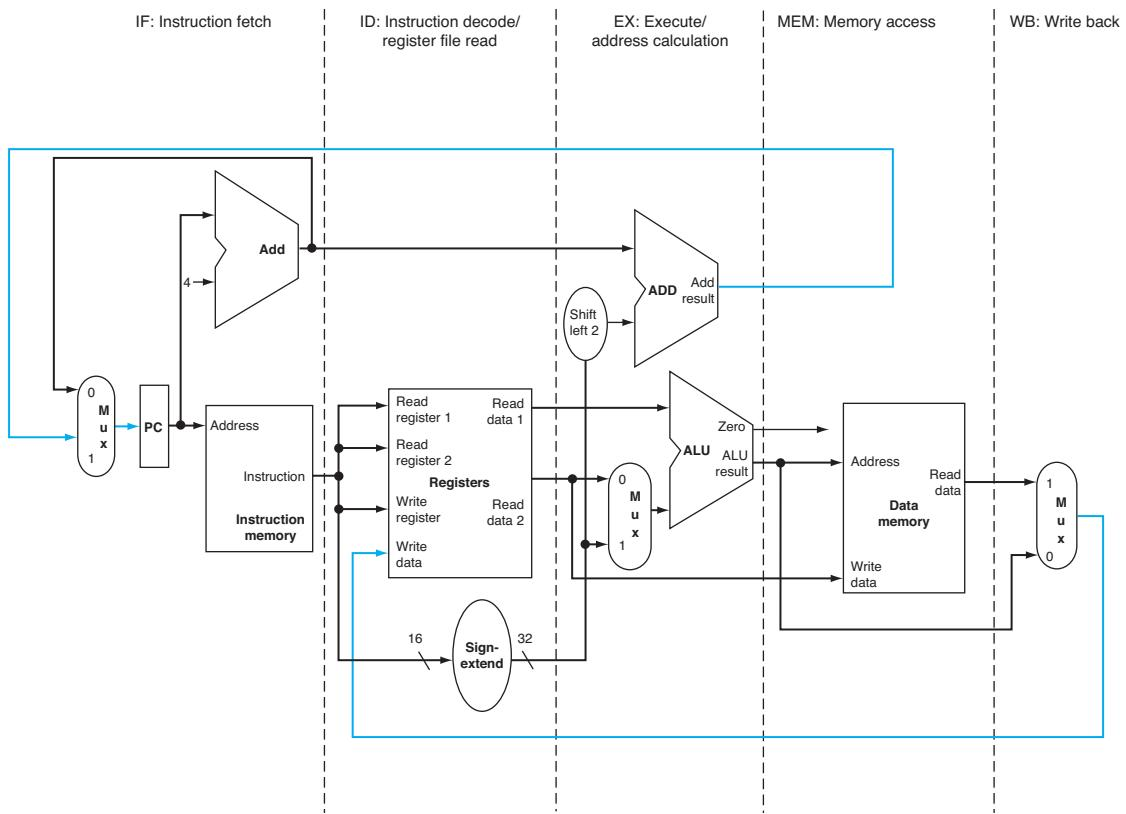
**FIGURE 4.33 The single-cycle datapath from Section 4.4 (similar to Figure 4.17).** Each step of the instruction can be mapped onto the datapath from left to right. The only exceptions are the update of the PC and the write-back step, shown in color, which sends either the ALU result or the data from memory to the left to be written into the register file. (Normally we use color lines for control, but these are data lines.)
