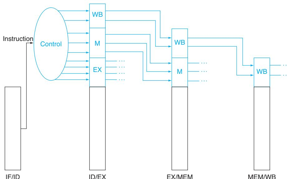
**FIGURE 4.50 The control lines for the final three stages.** Note that four of the nine control lines are used in the EX phase, with the remaining five control lines passed on to the EX/MEM pipeline register extended to hold the control lines; three are used during the MEM stage, and the last two are passed to MEM/WB for use in the WB stage.
