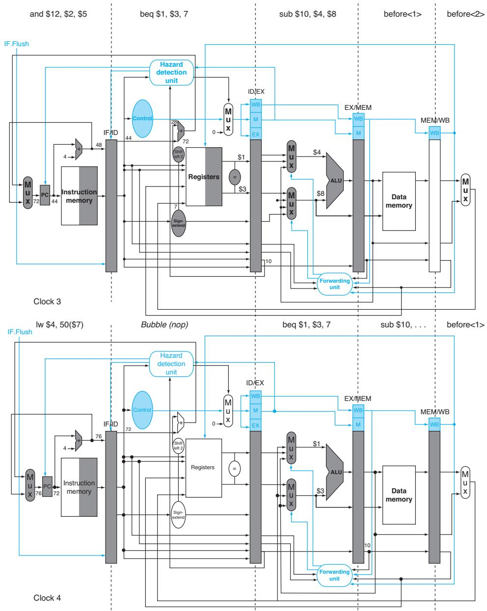
**FIGURE 4.62 The ID stage of clock cycle 3 determines that a branch must be taken, so it selects 72 as the next PC address and zeros the instruction fetched for the next clock cycle.** Clock cycle 4 shows the instruction at location 72 being fetched and the single bubble or nop instruction in the pipeline as a result of the taken branch. (Since the nop is really  $sll \$0, \$0, 0$ , it's arguable whether or not the ID stage in clock 4 should be highlighted.)
