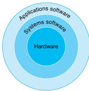
**FIGURE 1.2 A simplified view of hardware and software as hierarchical layers, shown as concentric circles with hardware in the center and applications software outermost.** In complex applications, there are often multiple layers of application software as well. For example, a database system may run on top of the systems software hosting an application, which in turn runs on top of the database.
