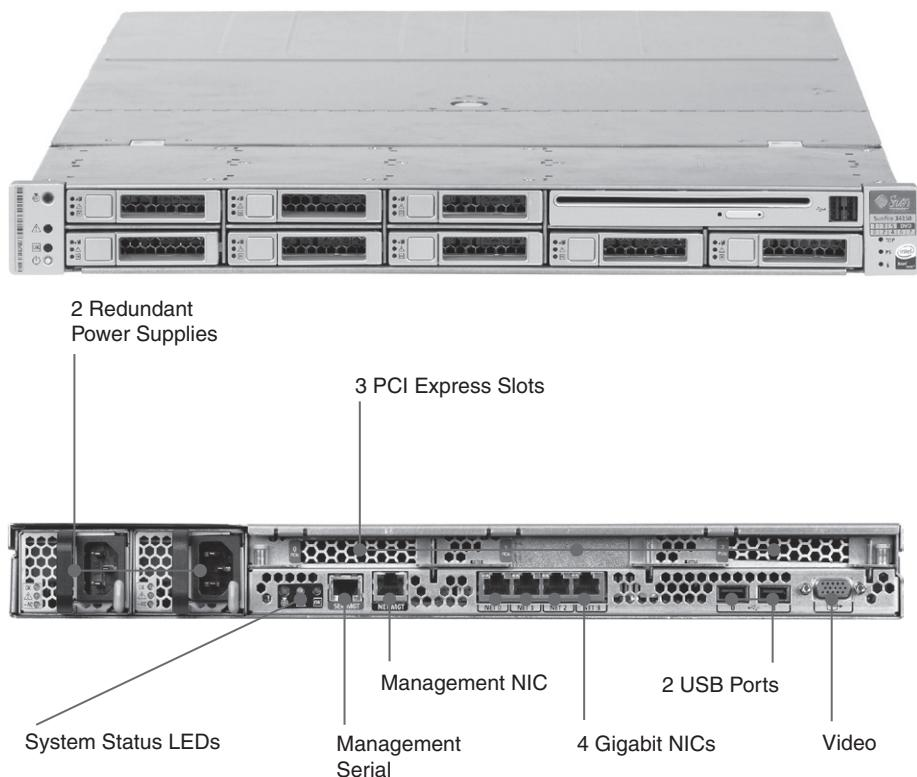
**FIGURE 6.16 The front and rear of the Sun Fire x4150 1U server.** The dimensions are 1.75 inches high by 19 inches wide. The eight 2.5-inch disks drives can be replaced from the front. In the upper right is a DVD and two USB ports. The picture below labels the items at the rear of the server. It has redundant power supplies and fans to allow the server to continue operating despite failures of one of these components.
