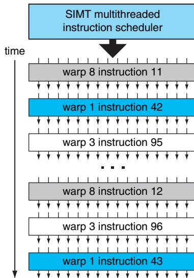
**FIGURE A.4.2 SIMT multithreaded warp scheduling.** The scheduler selects a ready warp and issues an instruction synchronously to the parallel threads composing the warp. Because warps are independent, the scheduler may select a different warp each time.
