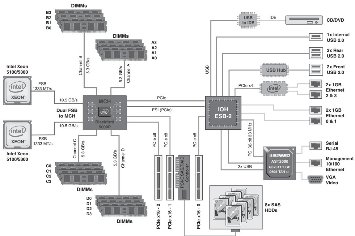
**FIGURE 6.17 Logical connections and bandwidths of components in the Sun Fire x4150.** The three PCIe connectors allow x16 boards to be plugged in, but it only provides eight lanes of bandwidth to the MCH. Source: Figure 5 of “SUN FIRE™ X4150 AND X4450 SERVER ARCHITECTURE” (see [www.sun.com/servers/x64/x4150/](http://www.sun.com/servers/x64/x4150/)).
