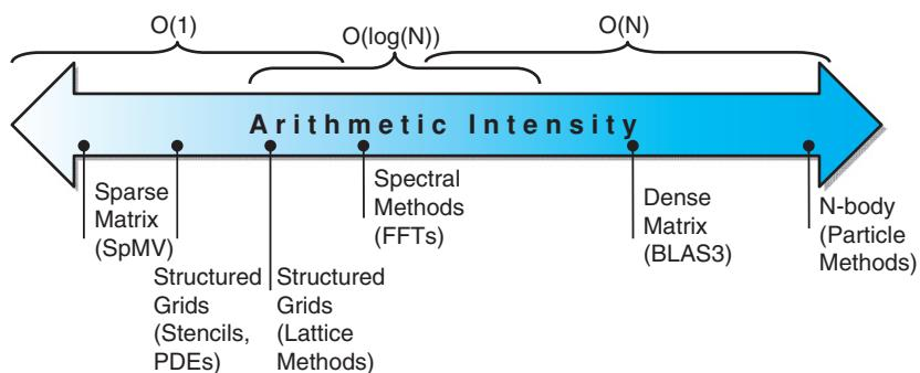
**FIGURE 7.12 Arithmetic intensity, specified as the number of float-point operations to run the program divided by the number of bytes accessed in main memory [Williams, Patterson, 2008].** Some kernels have an arithmetic intensity that scales with problem size, such as Dense Matrix, but there are many kernels with arithmetic intensities independent of problem size. For kernels in this former case, weak scaling can lead to different results, since it puts much less demand on the memory system.
