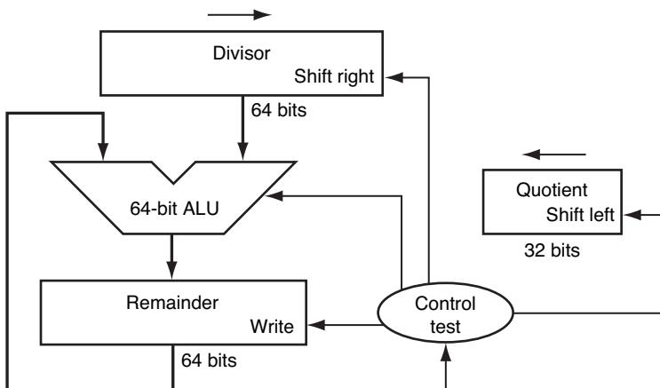
**FIGURE 3.9 First version of the division hardware.** The Divisor register, ALU, and Remainder register are all 64 bits wide, with only the Quotient register being 32 bits. The 32-bit divisor starts in the left half of the Divisor register and is shifted right 1 bit each iteration. The remainder is initialized with the dividend. Control decides when to shift the Divisor and Quotient registers and when to write the new value into the Remainder register.
