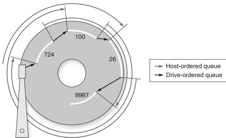
**FIGURE 6.19 Example showing OS versus disk schedule accesses, labeled host-ordered versus drive-ordered.** The former takes three revolutions to complete the four reads, while the latter completes them in just three-fourths of a revolution (from Anderson [2003]).
