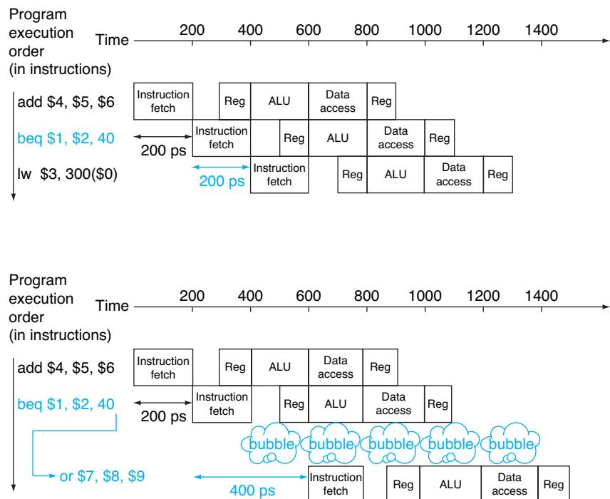
**FIGURE 4.32 Predicting that branches are not taken as a solution to control hazard.** The top drawing shows the pipeline when the branch is not taken. The bottom drawing shows the pipeline when the branch is taken. As we noted in Figure 4.31, the insertion of a bubble in this fashion simplifies what actually happens, at least during the first clock cycle immediately following the branch. Section 4.8 will reveal the details.
