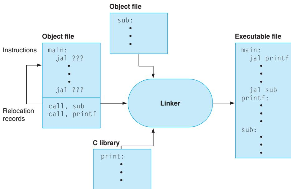
**FIGURE B.3.1** The linker searches a collection of object files and program libraries to find nonlocal routines used in a program, combines them into a single executable file, and resolves references between routines in different files.
