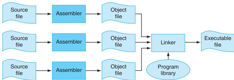
**FIGURE B.1.1** The process that produces an executable file. An assembler translates a file of assembly language into an object file, which is linked with other files and libraries into an executable file.
