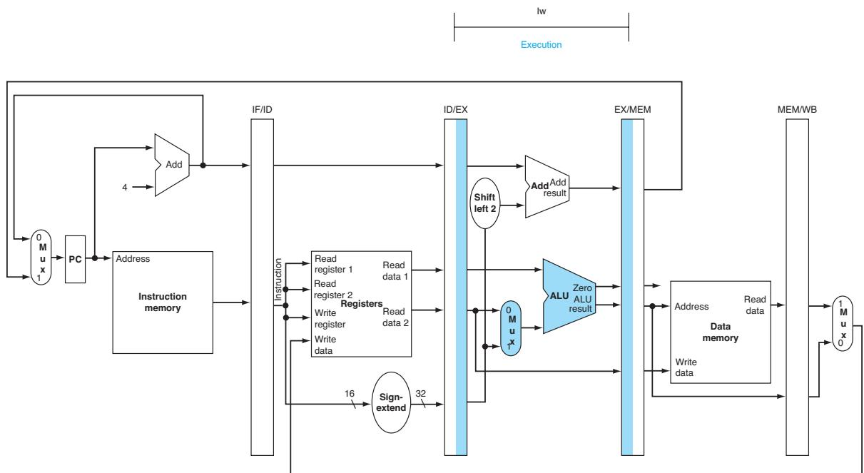
**FIGURE 4.37 EX: The third pipe stage of a load instruction, highlighting the portions of the datapath in Figure 4.35 used in this pipe stage.** The register is added to the sign-extended immediate, and the sum is placed in the EX/MEM pipeline register.
