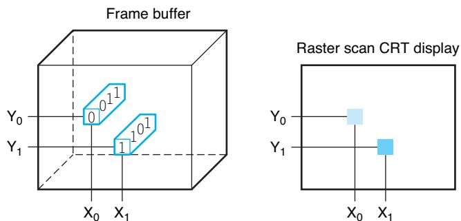
**FIGURE 1.6** Each coordinate in the frame buffer on the left determines the shade of the corresponding coordinate for the raster scan CRT display on the right. Pixel  $(X_0, Y_0)$  contains the bit pattern 0011, which is a lighter shade on the screen than the bit pattern 1101 in pixel  $(X_1, Y_1)$ .
