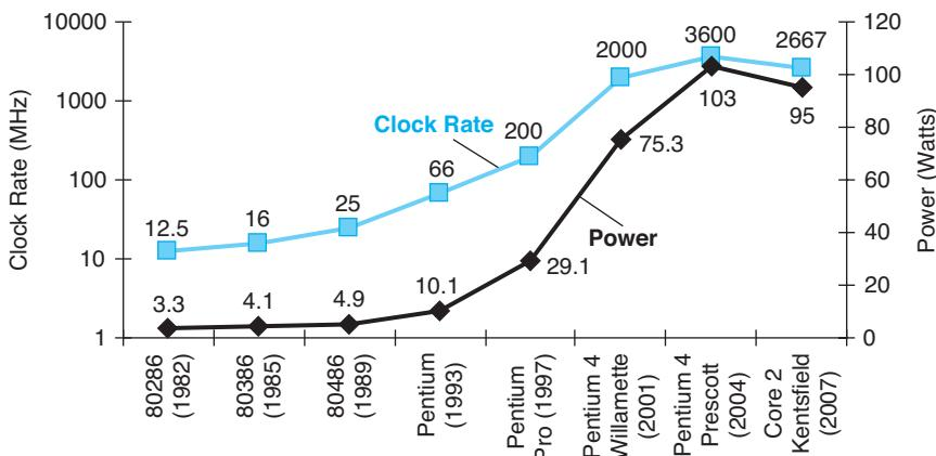
**FIGURE 1.15 Clock rate and Power for Intel x86 microprocessors over eight generations and 25 years.** The Pentium 4 made a dramatic jump in clock rate and power but less so in performance. The Prescott thermal problems led to the abandonment of the Pentium 4 line. The Core 2 line reverts to a simpler pipeline with lower clock rates and multiple processors per chip.
