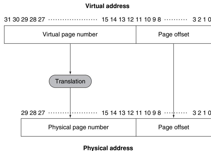
**FIGURE 5.20 Mapping from a virtual to a physical address.** The page size is  $2^{12} = 4$  KB. The number of physical pages allowed in memory is  $2^{18}$ , since the physical page number has 18 bits in it. Thus, main memory can have at most 1 GB, while the virtual address space is 4 GB.
