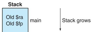
**Elaboration:** The difference between the MIPS compiler and the gcc compiler is that the MIPS compiler usually does not use a frame pointer, so this register is available as another callee-saved register, `$s8`. This change saves a couple of instructions in the procedure call and return sequence. However, it complicates code generation, because a procedure must access its stack frame with `$sp`, whose value can change during a procedure's execution if values are pushed on the stack.
