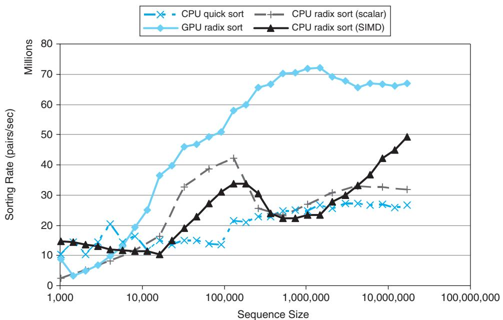
**FIGURE A.7.6 Parallel sorting performance.** This graph compares sorting rates for parallel radix sort implementations on a 1.5 GHz GeForce 8800 Ultra and an 8-core 2.33 GHz Intel Core2 Xeon E5345 system.
