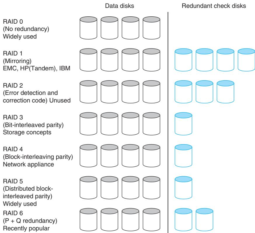
**FIGURE 6.12 RAID for an example of four data disks showing extra check disks per RAID level and companies that use each level.** Figures 6.13 and 6.14 explain the difference between RAID 3, RAID 4, and RAID 5.
