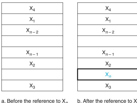
**FIGURE 5.4 The cache just before and just after a reference to a word  $X_n$  that is not initially in the cache.** This reference causes a miss that forces the cache to fetch  $X_n$  from memory and insert it into the cache.
