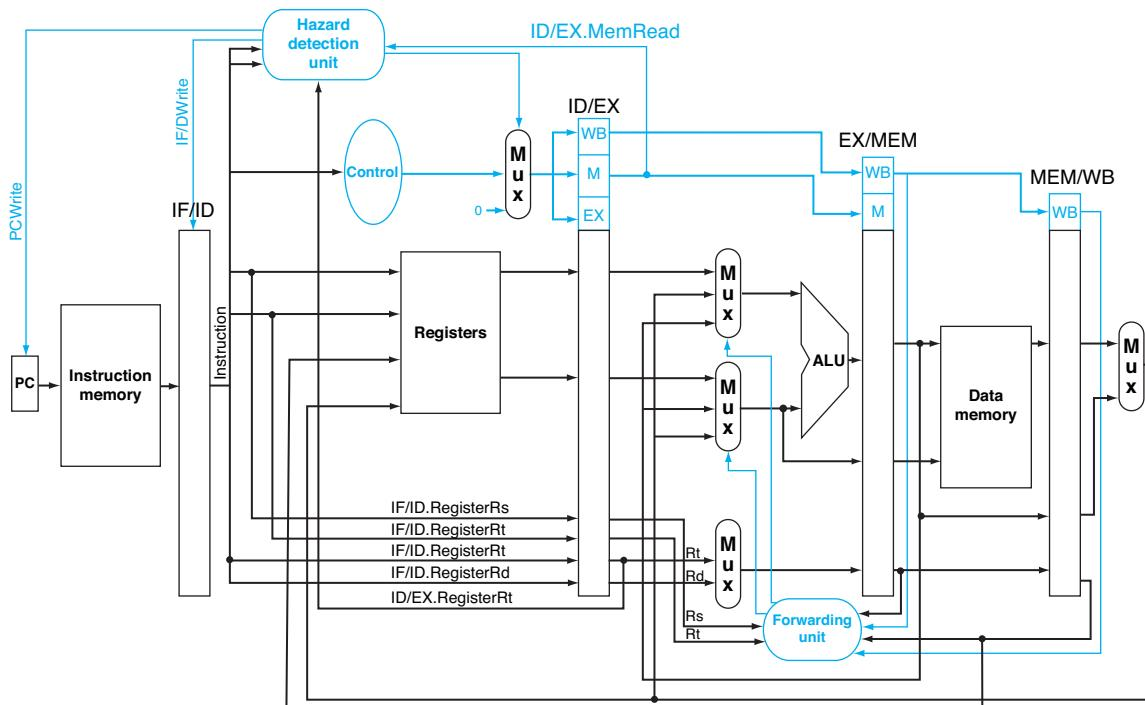
**FIGURE 4.60 Pipelined control overview, showing the two multiplexors for forwarding, the hazard detection unit, and the forwarding unit.** Although the ID and EX stages have been simplified—the sign-extended immediate and branch logic are missing—this drawing gives the essence of the forwarding hardware requirements.
