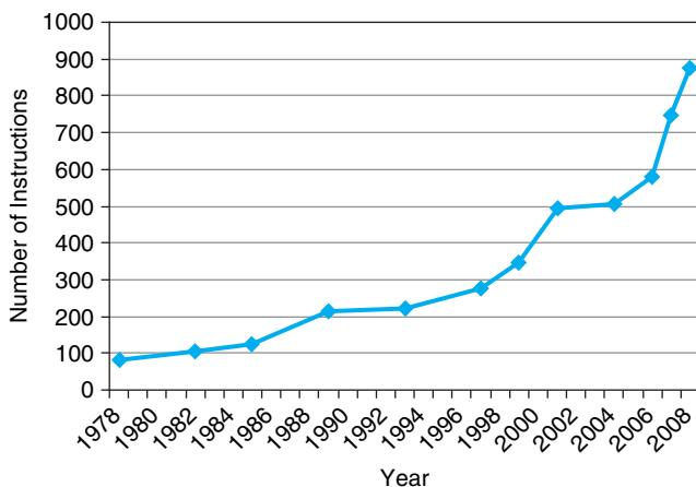
**FIGURE 2.43 Growth of x86 instruction set over time.** While there is clear technical value to some of these extensions, this rapid change also increases the difficulty for other companies to try to build compatible processors.
