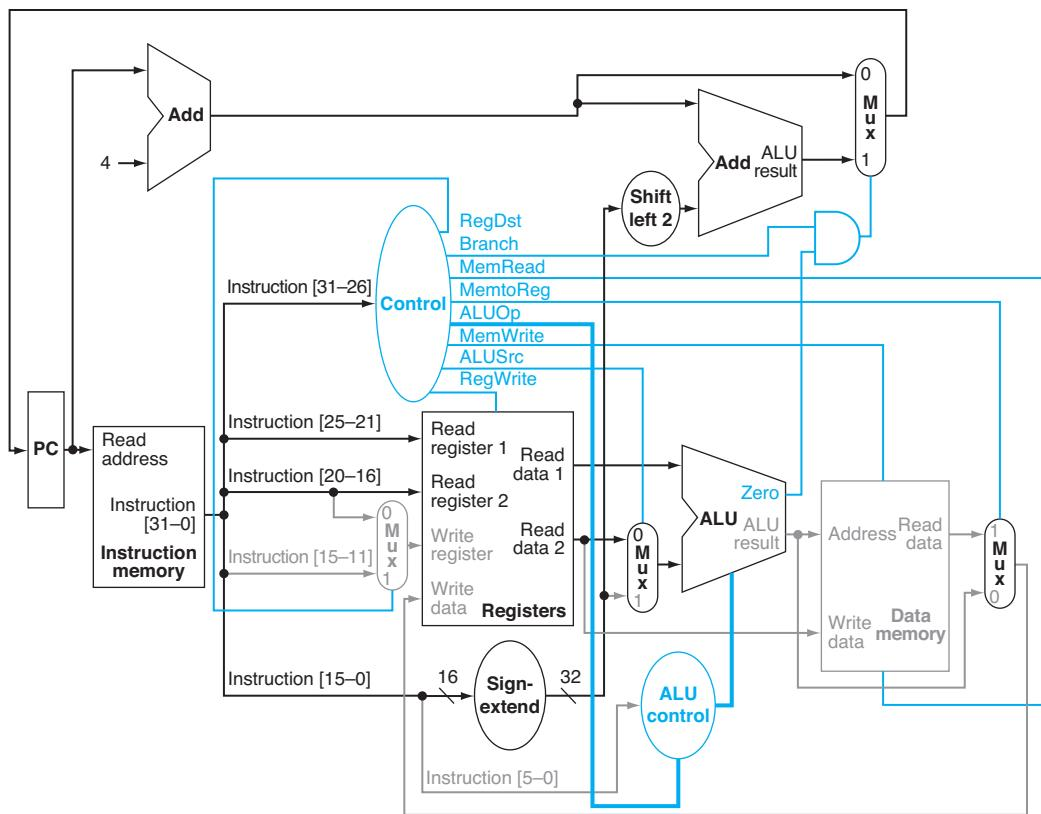
**FIGURE 4.21** The datapath in operation for a branch-on-equal instruction. The control lines, datapath units, and connections that are active are highlighted. After using the register file and ALU to perform the compare, the Zero output is used to select the next program counter from between the two candidates.
