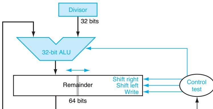
**FIGURE 3.12 An improved version of the division hardware.** The Divisor register, ALU, and Quotient register are all 32 bits wide, with only the Remainder register left at 64 bits. Compared to Figure 3.9, the ALU and Divisor registers are halved and the remainder is shifted left. This version also combines the Quotient register with the right half of the Remainder register. (As in Figure 3.6, the Remainder register should really be 65 bits to make sure the carry out of the adder is not lost.)
