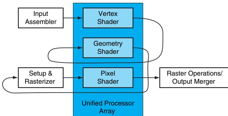
**FIGURE A.2.4 Logical pipeline mapped to physical processors.** The programmable shader stages execute on the array of unified processors, and the logical graphics pipeline dataflow recirculates through the processors.
