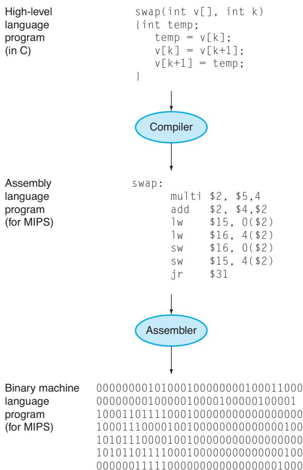
**FIGURE 1.3 C program compiled into assembly language and then assembled into binary machine language.** Although the translation from high-level language to binary machine language is shown in two steps, some compilers cut out the middleman and produce binary machine language directly. These languages and this program are examined in more detail in Chapter 2.
