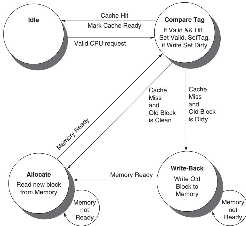
FIGURE 5.34 Four states of the simple controller.
