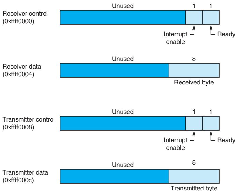
**FIGURE B.8.1 The terminal is controlled by four device registers, each of which appears as a memory location at the given address.** Only a few bits of these registers are actually used. The others always read as 0s and are ignored on writes.
