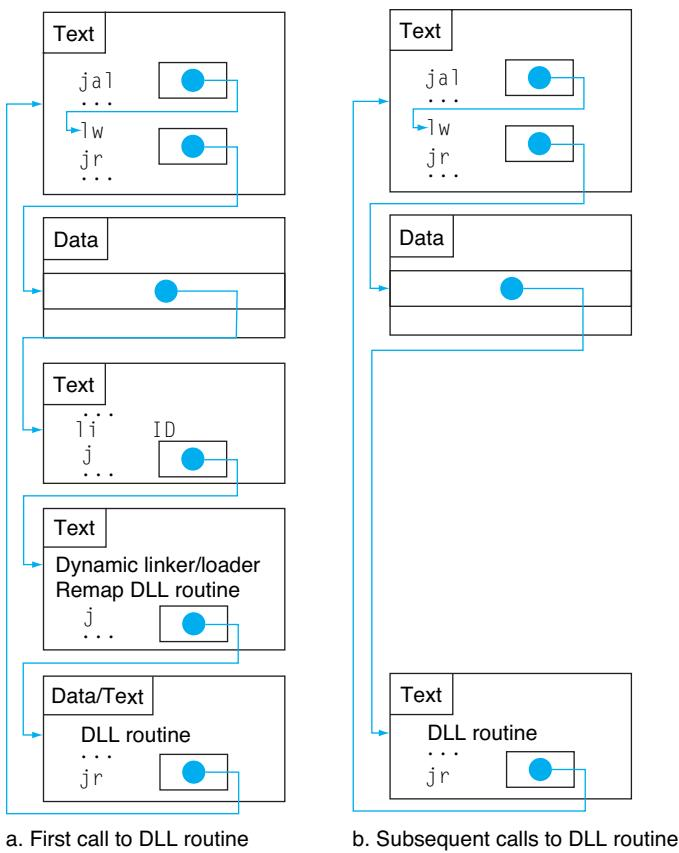
**FIGURE 2.22** **Dynamically linked library via lazy procedure linkage.** (a) Steps for the first time a call is made to the DLL routine. (b) The steps to find the routine, remap it, and link it are skipped on subsequent calls. As we will see in Chapter 5, the operating system may avoid copying the desired routine by remapping it using virtual memory management.
