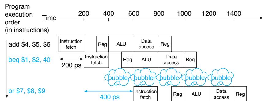
**FIGURE 4.31 Pipeline showing stalling on every conditional branch as solution to control hazards.** This example assumes the conditional branch is taken, and the instruction at the destination of the branch is the `OR` instruction. There is a one-stage pipeline stall, or bubble, after the branch. In reality, the process of creating a stall is slightly more complicated, as we will see in [Section 4.8](#). The effect on performance, however, is the same as would occur if a bubble were inserted.
