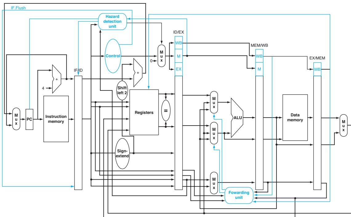
**FIGURE 4.65** The final datapath and control for this chapter. Note that this is a stylized figure rather than a detailed datapath, so it's missing the ALUsrc mux from Figure 4.57 and the multiplexer controls from Figure 4.51.
